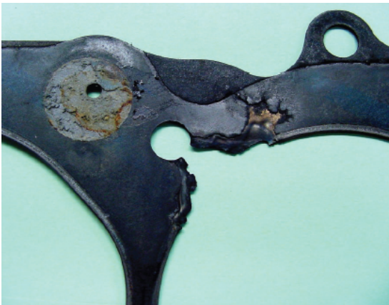
Figure 1: Detonation has distorted the combustion seal and gases escape into the cooling system.
