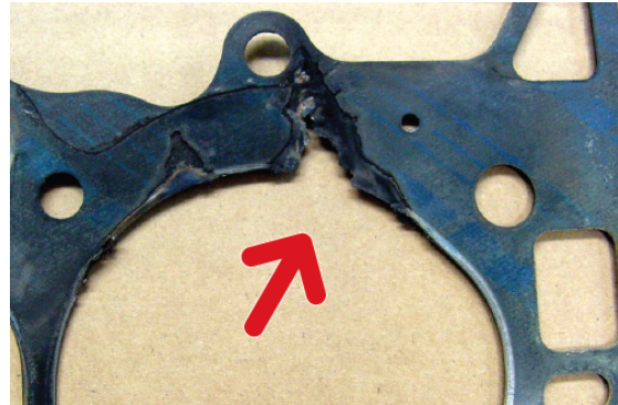
Figure 2: Excessive pressure waves eventually burned through the gasket.
